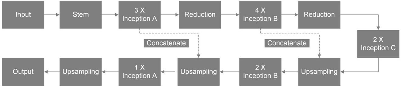
**Fig. 3.** The network architecture of the proposed semantic segmentation network based on inception structures.
